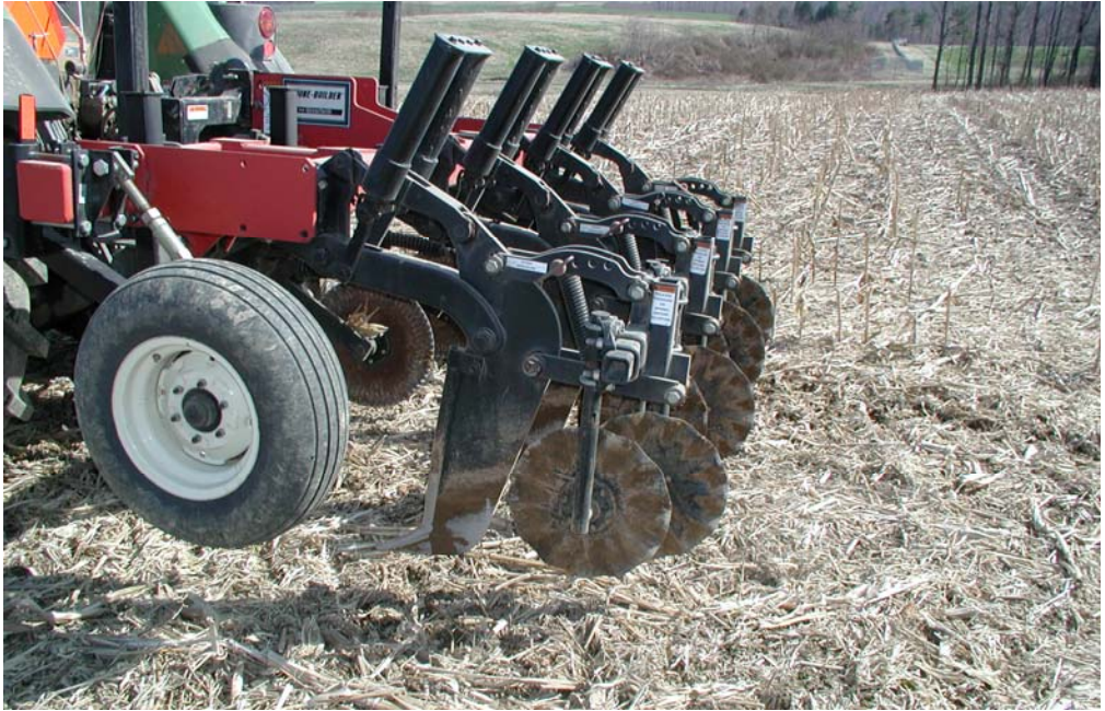
Figure 6.8. Two types of modern subsoilers that break through subsoil compaction while conserving surface residue cover.
